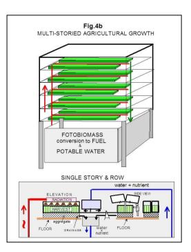
**Fig.4b** illustrates schematically a space saving and highly automated system for the same photosynthesising purposes.
